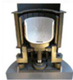
CZ Furnace for single crystal silicon manufacturing
