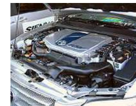
Toyota FCHV PEM FC fuel cell vehicle
