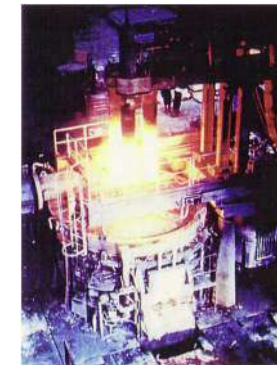
Iron Smelting in Electric Arc Furnace. Needle Coke Electrode.
